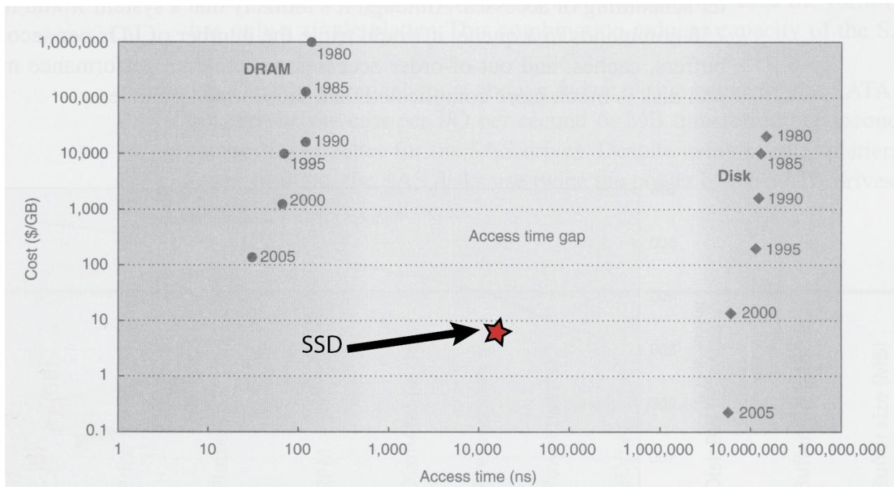
The star representing the STEC SSD is placed on the chart by hand, approximately in the correct location in terms of access time. I have not paid much attention to the cost axis, but it is very roughly correct as far as I can determine. This shows that the current generation of SSD devices have very successfully closed the access time gap. As the pricing drops further, the cost/GB will eventually become lower than even magnetic media — this is a very significant event in database processing.
