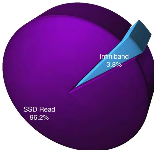
The application of Infiniband makes sense for this reason: It returns the overhead of the interconnect back to the relative levels we are used to with Fibre Channel and magnetic disk.
