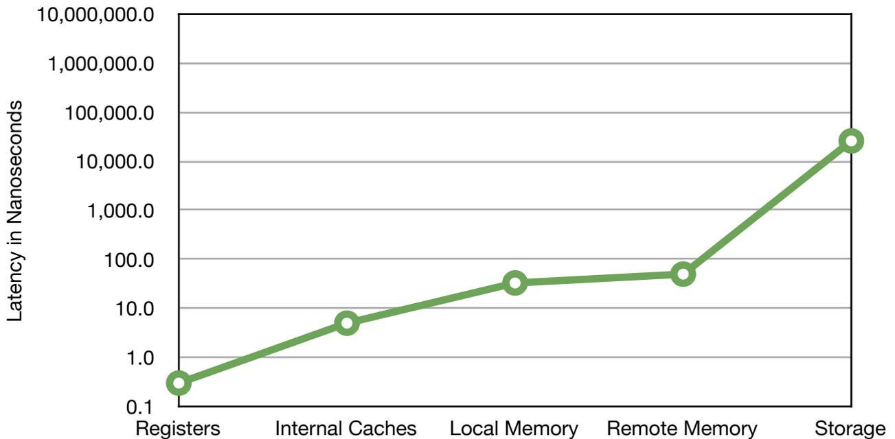
This is really just another way at looking at the ‘access time gap’ defined in [HENN 2007], but applied to the whole memory hierarchy. It shows that the memory hierarchy has moved from a span of eight orders of magnitude to only five, even when looking all the way back to the registers.
