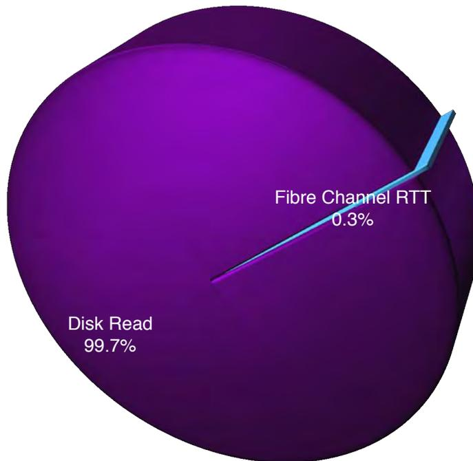
There is no problem evident when using Fibre Channel in this configuration; the disk latencies are so high that the Fibre Channel latency is minimal. There would be no benefit at all seen from using IB in this configuration from a latency standpoint, though there could still be one for reasons of bandwidth.
