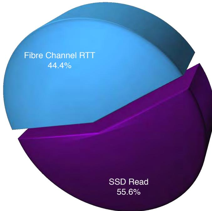
As you can clearly see, the overhead of the Fibre Channel latency is now a significant factor in the total latency of the read operation. Please note that the Fibre Channel time has not *increased*, but rather the proportion of total I/O time has increased because the I/O time has reduced so much.
