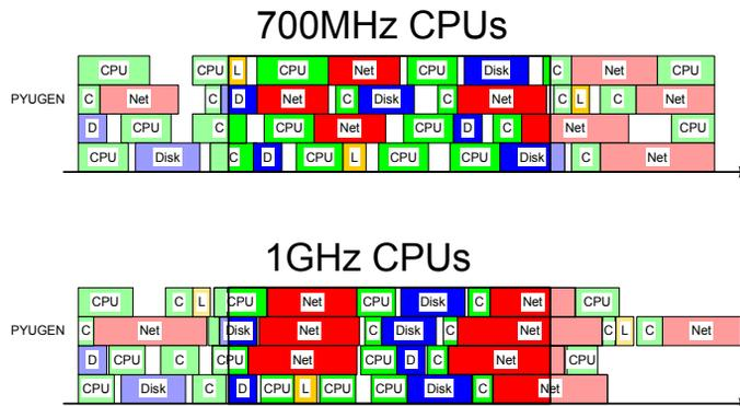
Queueing theory predicts that, on a busy system, an upgrade to a component that is not **your** bottleneck can cause performance degradation for you. The picture here shows how. By upgrading to faster CPUs, all the CPU service durations get smaller. However, because before the upgrade PYUGEN spends only about 18% of its time consuming the CPU resource, the CPU upgrade does not provide much elapsed time benefit to PYUGEN.
